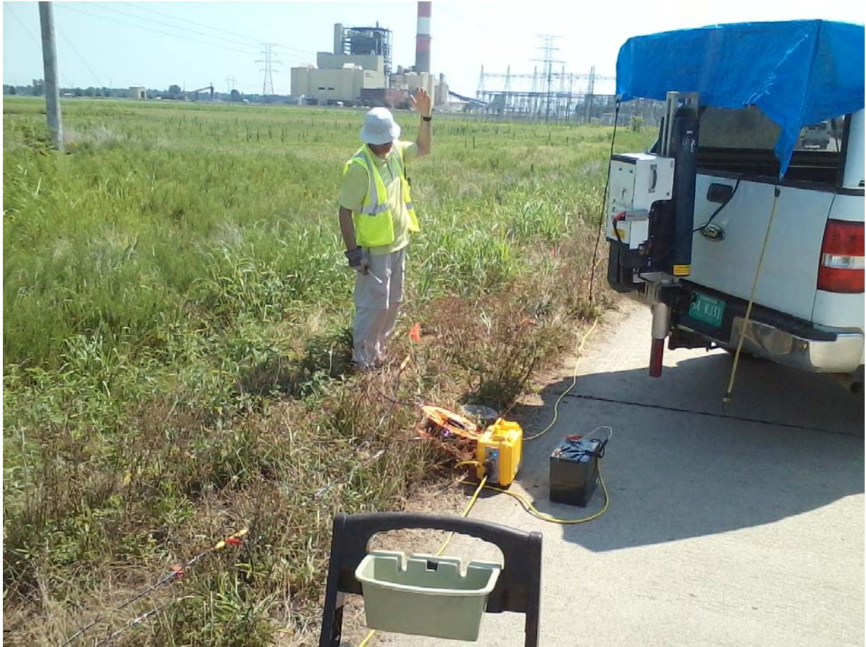
Figure 2: Picture of the MASW survey being conducted next to the road with the power plant in the background.
